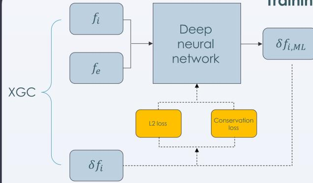
$$L_{L2} = \frac{1}{n} \sum_{i=1}^n (\delta f_{XGC} - \delta f_{ML})^2 \quad L_{cons} = \sum_{i=1}^3 \lambda_i (x^i \delta f_{XGC} - x^i \delta f_{ML})$$
